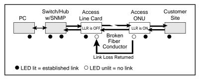
*Important: LLR must not be active on both ends of a configuration. If it is, the link can never be established.*
